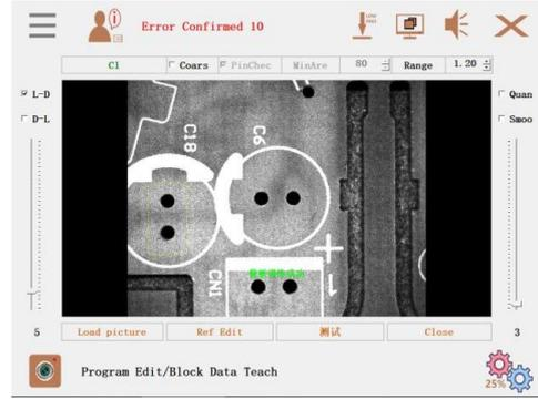
d. Click **【 The edit characteristics】** into the interface, based on green text, and then the right mouse button to choose start point and end point (note: the starting point and destination choice needs corresponding element to identify the direction, so please keep in mind that the current setting), back to the main screen click **【 recognition test】** prompts recognition success click **【 teach photograph position】** saves the current coordinates.
