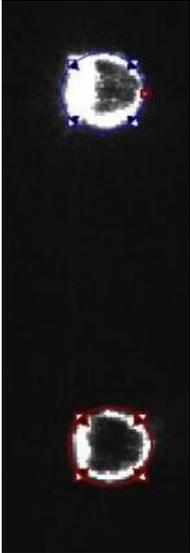
h. Select the starting point and ending point, right-click the mouse and choose **【 Set Starting point】** & **【 Set End point】** (note: the selection needs to correspond to the starting point and end point of the insert hole in **【 Block Data】** ). If the setting is successful, there will be change the color and the interface will be closed
